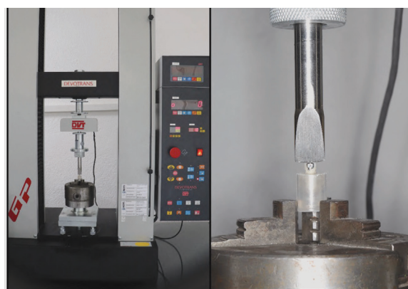
Fig. 2 Shear bond strength analysis with a universal testing machine.
